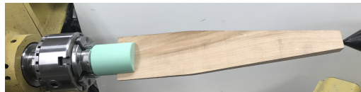
In your Scroll Chuck with jaws that close to at least 1 ½ inches.
