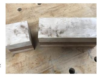
Make sure to cut the body to size on the OPPOSITE end from where you cut the head. This keeps the grain pattern consistent between the body and head.
