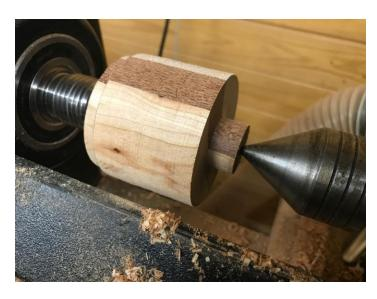
Mount the head blank with the 'T' at headstock and 'B' at live center - Spindle turn between centers to round.
