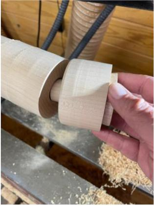
TEST FIT THE HEAD at this point. The head inset tenon should fit cleanly into the 1-1/16" hole of the body with no slop or play.
