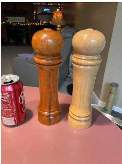
If using Parfix 3408 as your finish and doing it on the lathe, remove the head from body first. You don't want to accidentally glue the head to the body. Apply 3408 to the head by hand. This also gives you the opportunity to 3408 the top of the body and the bottom of the head now that they are separated.
