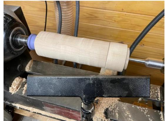
Turn/shape/sand/finish. Don't forget to sand the bottom.
