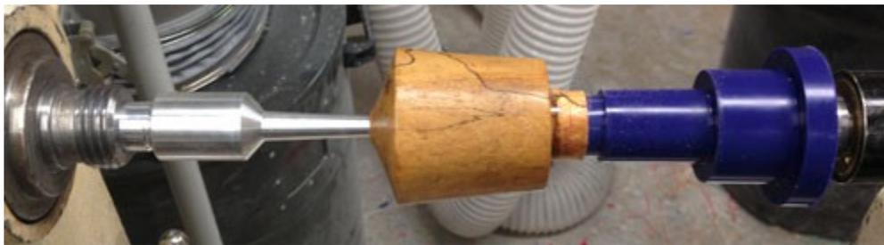
The arbor and one of the purple chuckies can hold the top and bottom of the pepper mill simultaneously.
