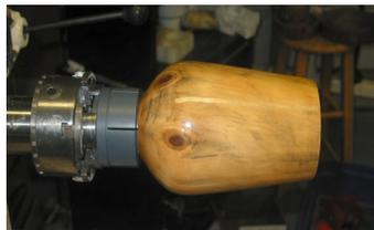
For different size holes, simply slip the appropriate ring onto the base unit and expand the rings. The 1" Expansion Chucky allows for hole openings of 1" through 1 7/8" while the 2" allows for holes from 2" through 2 7/8". These sizes are in 1/8" increments.
