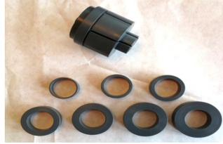
They can be used for many items and are adjustable in two ways; by turning the Hex Bolt from the front or rear of the Expansion Chucky.
