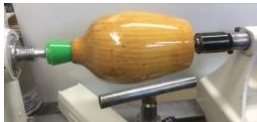
Hollow Form mounted on Chucky Arbor and Live Center
