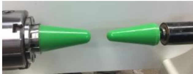
Mounted in Scroll Chuck and Live Center
