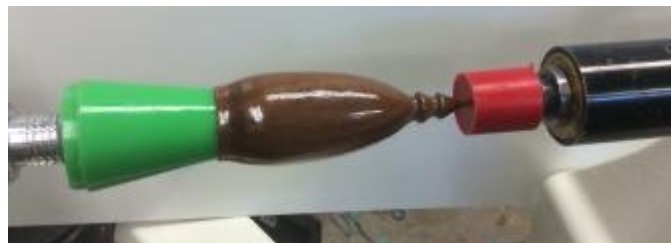
Hollow Form mounted on Chucky Arbor and Live Center
