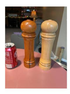
If using Parfix 3408 as your finish and doing it on the lathe, remove the head from body first. You don't want to accidently glue the head to the body. Apply 3408 to the head by hand. This also gives you the opportunity to 3408 the top of the body and the bottom of the head now that they are separated.
