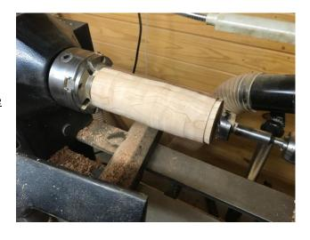
True up the edge and face of the tenon on the 'B' end now. This ensures the tenon is now turned true to the hole you just drilled. Skipping this step will result in alignment issues later.
