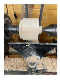
Mount the head blank with the 'T' at headstock and 'B' at live center - Spindle turn between centers to round.
