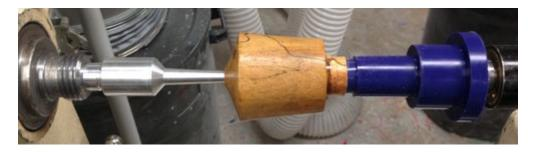
The arbor and one of the purple chuckies can hold the top and bottom of the pepper mill simultaneously.
